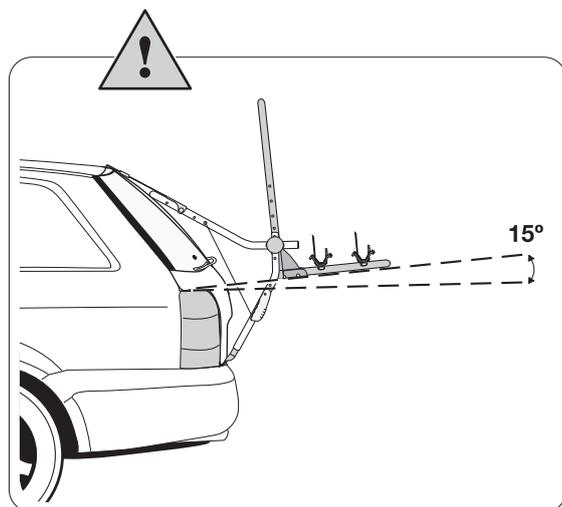
**EN** Select the right height and holes for installation. The platform should not obstruct the rear lights or number plate.
