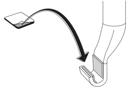
**EN** Check that the hooks remain free when shut. If the lower hooks strike the bumper, the rubber protector can be split and fitted on the sides of the lower hooks.
